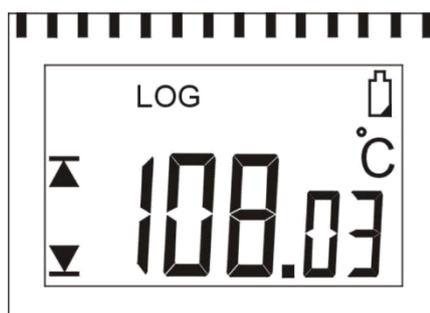
Appearing on display only battery symbol means logger does not work and battery has to be changed.
