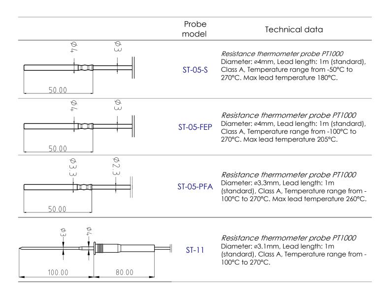
We are able to make probes with different lead length, probe length, probe diameter and sensors like PT100/PT500 depending on your needs.
