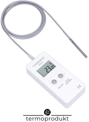
DT-1 and DT-2 thermometers are intended for measuring temperatures in the range of -50°C to 270°C. The devices are equipped with a measurement probe containing PT 1000 sensor. Example usage: measuring the temperature in food industry, laboratories, refrigerators or cold rooms.
