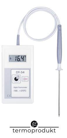
DT-34 thermometer is intended for measuring temperatures in the range of -100°C to 270°C. The devices are equipped with a measurement probe containing PT 1000 sensor. Example usage: measuring the temperature in food industry, laboratories, refrigerators or cold rooms.
